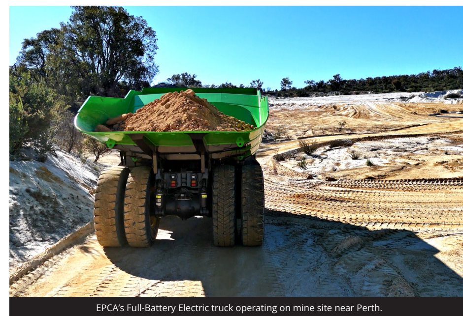
EPCA's Full-Battery Electric truck operating on mine site near Perth.
